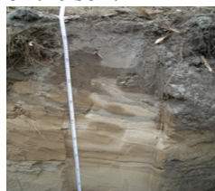
Plate 2. Water repellency: irregular wetting in the vertical soil profile in Block B after overnight rainfall of 108 mm
