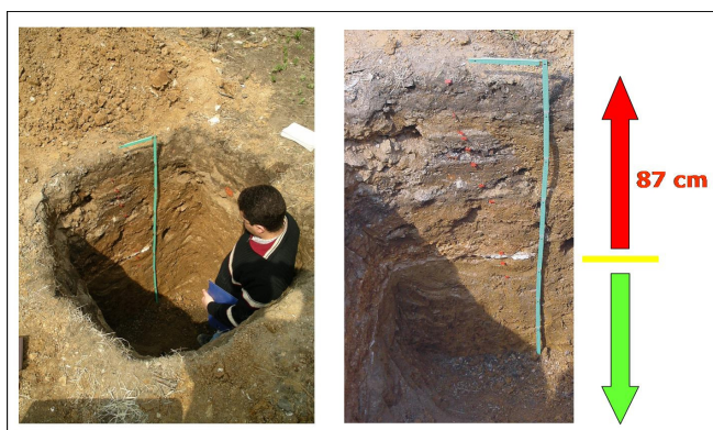
Figure 3. Technosol over capped Cambisol in the Old City of Qingdao. 87 cm of new material accumulated since the first construction development (indicated by the white band that is a lime terrace) took place during the German occupation about 100 years ago.
